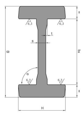
"H" shape milled profiles are obtained directly from "H" rolled profiles. The faces on which slide combined bearings are processed through the machine tool, obtaining an excellent degree of surface finishing together extremely small tolerances. This ensures absolute precision of a coupling between bearing and profile, reducing to limit the clearance between them, making it an excellent economical alternative to linear guides in trade.
